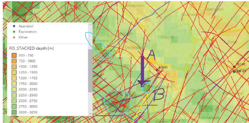
Figure 4 Snapshot from ThermoGIS of top Rotliegendes depth map in the Utrecht region. In red location of seismic lines, in purple location of seismic line MZ85-14 (partially shown in Figure 5) and section of DGM model v4.0 (Figure 6)
