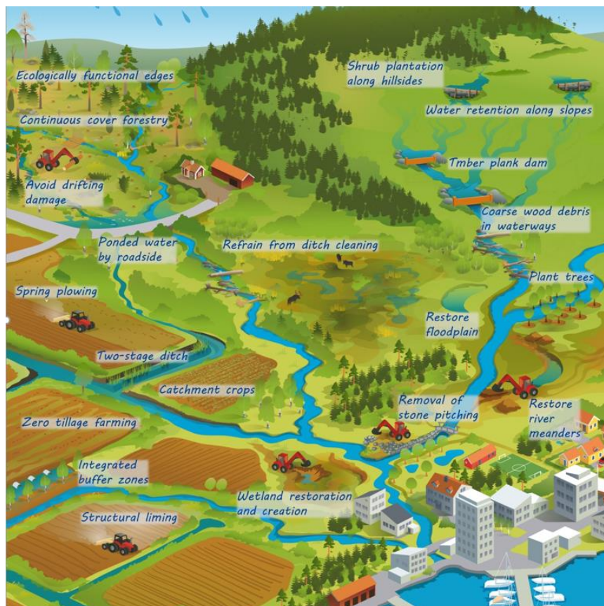
Figure 2.5 NBS for restoring flood risk in upper, middle and lower river sections. From Life IP Rich Waters
