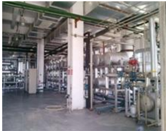
Figure 6-4: Photographs of compact zeolite membrane plants processing 1,000 to 3,000 gallons per day of wet ethanol [S24].
